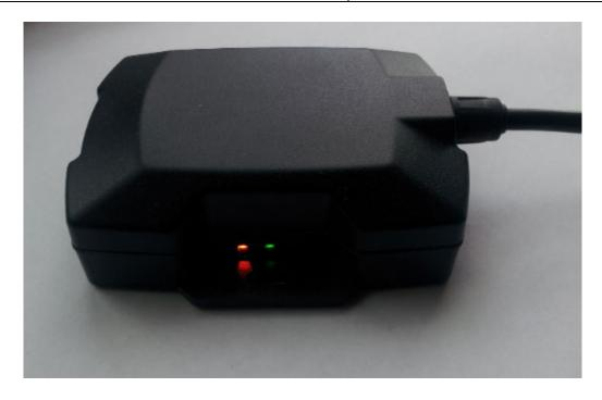
After the unit has been powered for 5 to 15 minutes, the unit will send in a "power-up" message.
